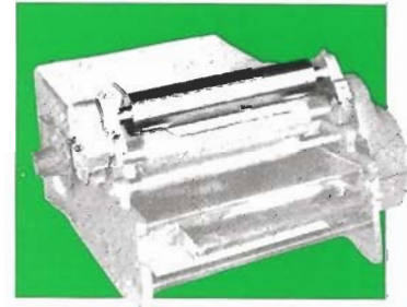
POTDEVIN Type 2R with CARDBOARD attachment. Display cards, advertising displays, mounts for photographs, lined cardboard, etc., can be produced rapidly and economically with POTDEVINS. Plywood, glass, and other rigid materials can also be coated with this attachment.
