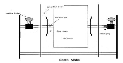
There are two 11" long, 1/16" aluminum roll guides and (1) tension spring included with the machine. These guides should be placed on either side of the roll of labels between the metal core inserts and the locking collar. The notches on the end of the guide slide onto the chrome rod at the bottom of the machine. One tension spring goes between the right roll guide and the locking collar on the right side of the roll of labels.
